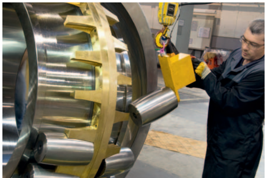
Schaeffler has produced an extraordinary spherical roller bearing for what is currently the world's largest roller press. The outside diameter is nearly two meters, and each roller weighs 50 kilograms.
