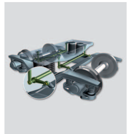
Track stabilisation, torsion bar
