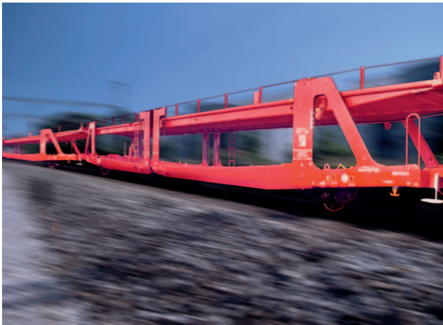
Twin level car transporter wagon Laes 559, Tatravagónka a.s
