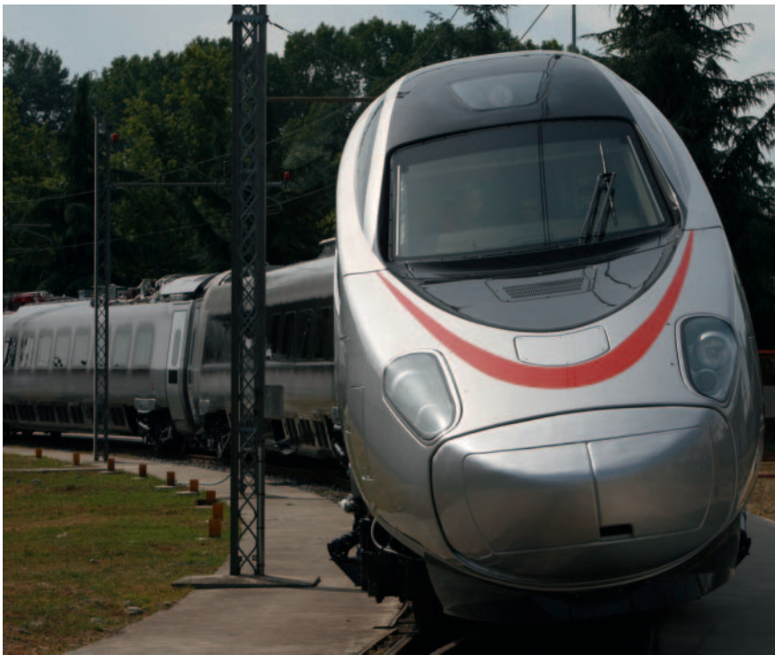
TR 600 (Trenitalia); ETR 610 (Cisalpio) with 4th generation tilting system
