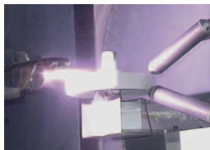
Plasma spraying method
