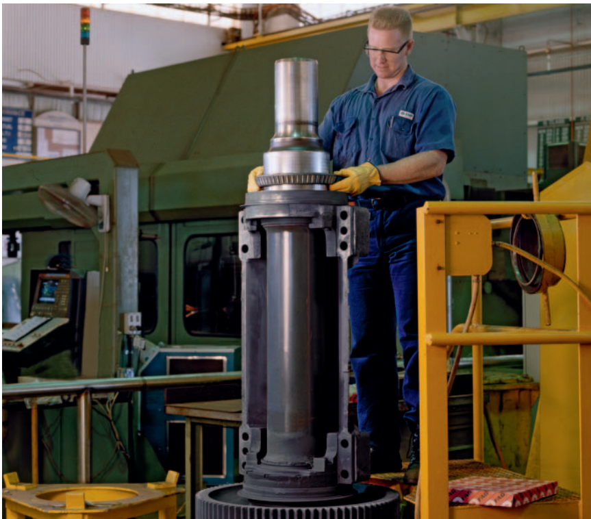
Mounting of nose and axle-suspended motor bearing
